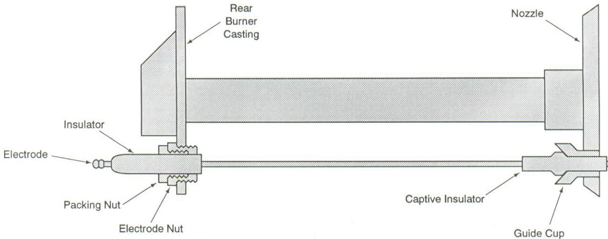
**The ignition plug and flame rod for sizes 50 through 600 are identical parts:**
