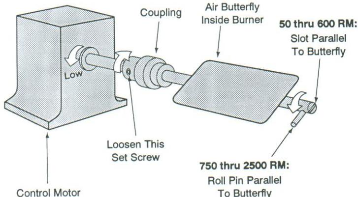
1. Drive the control motor to its low fire position.
